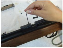
6. Tighten the set screws on the mount
