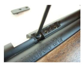
2. Remove the bolt cam screw from the bolt
